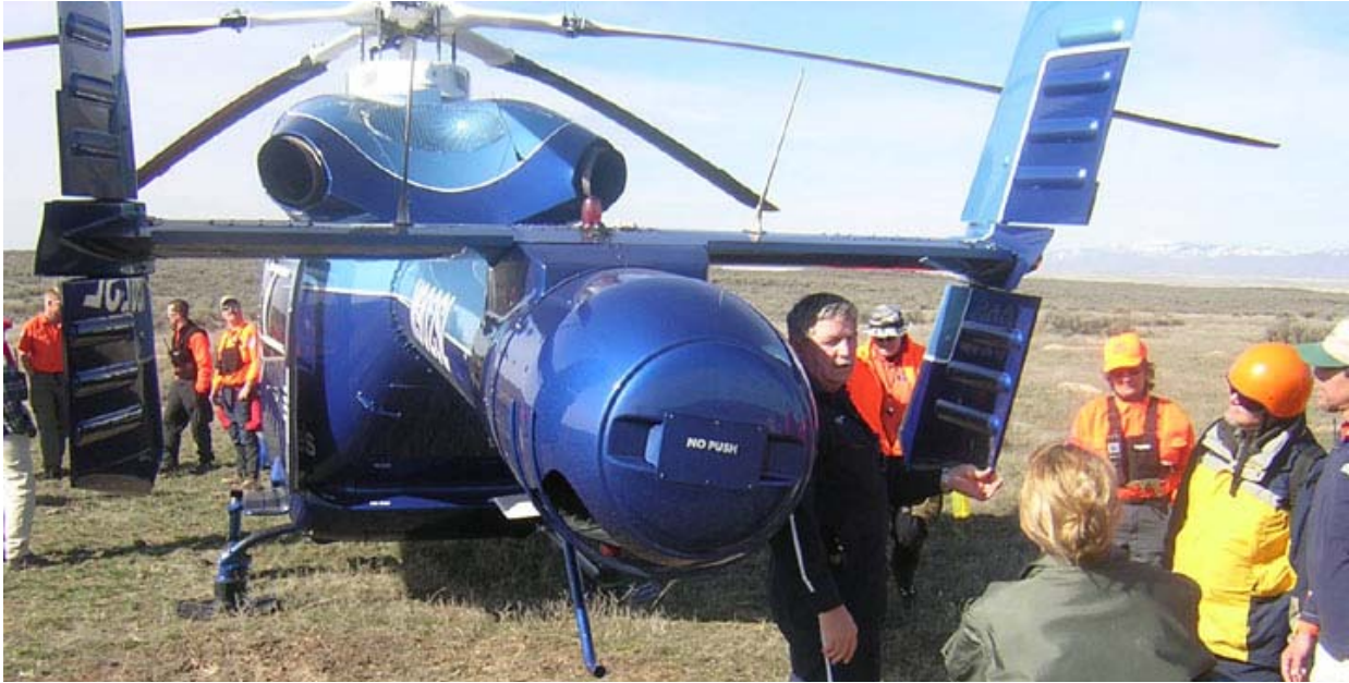
Look, no tail rotor! Air St. Luke's staff gives an orientation to their MD900.
