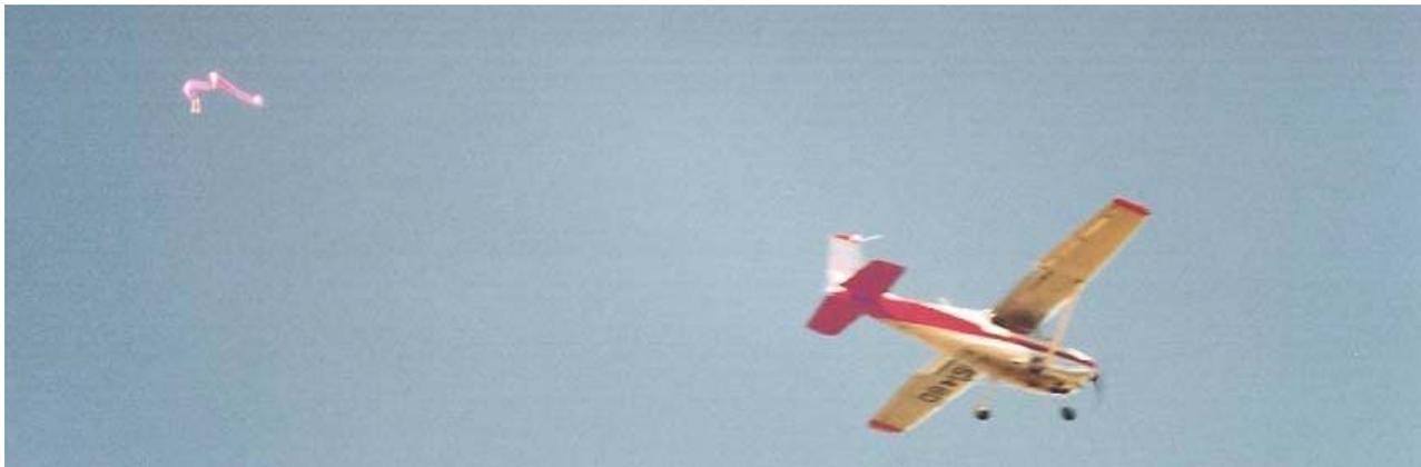
This plane has just released a cushiony case that contains a Family Service Radio for use by a “victim” on the ground. The streamer makes the package visible to the person who needs it.
