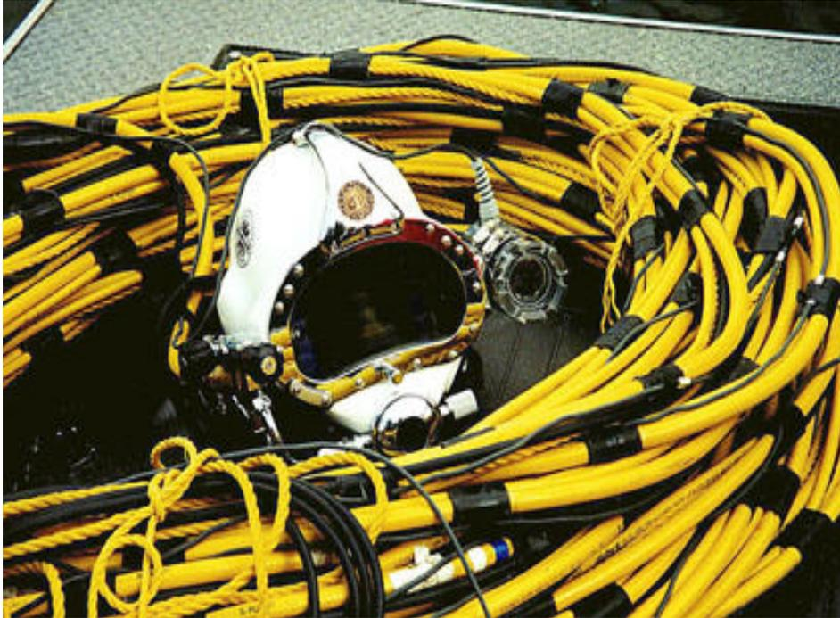
Dive helmet with TV camera and cable used for NITROX dives.
